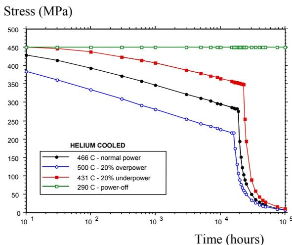
Fig. 3: Stress to failure variation with time, temperature and damage rate for various events
