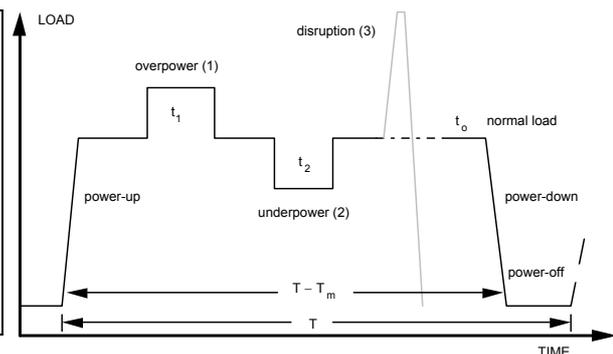
Fig. 2: A schematic of the loading histogram for in-vessel components event history.
